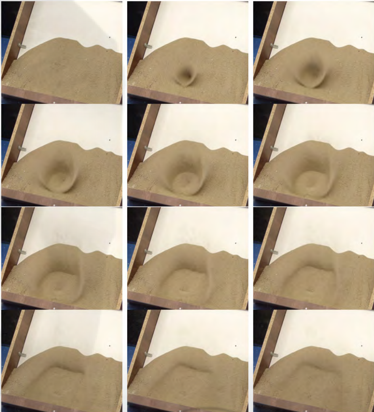
Figure 1 Panel Image Representing Different Consecutive Frames Due to the Penetration of the Projectile into the Substrate and a Few Moments After the Penetration
