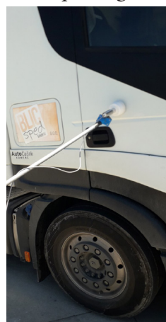
Figure 4. Ambient Dose Rate Equivalent Measurement on the Driver's Position
