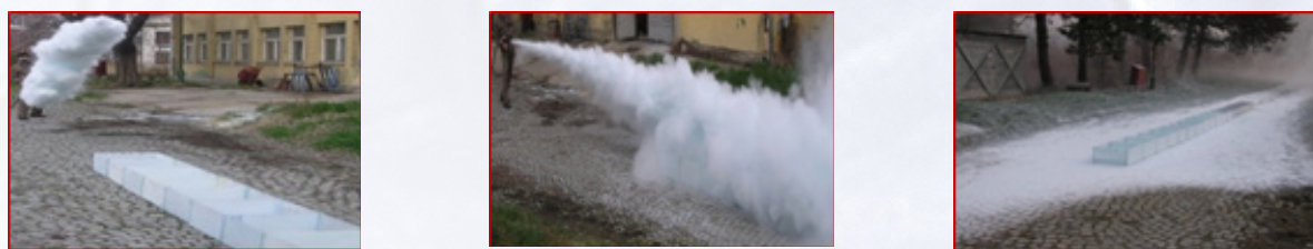
Figure 1 – Measuring jet range and time of continuous discharge
