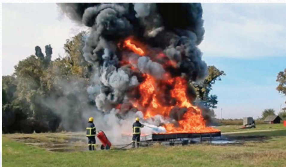
Figure 2 – Extinguishing fire at type B test fire
