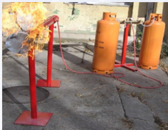
Figure 6 – Testing extinguishing at gas installations
